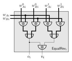
Figure 9. Circuit realization of EqualRev<sub>i</sub>.
