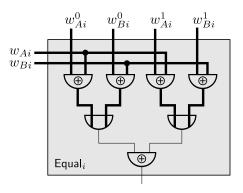
Figure 8. Circuit realization of  $Equal_i$ .
