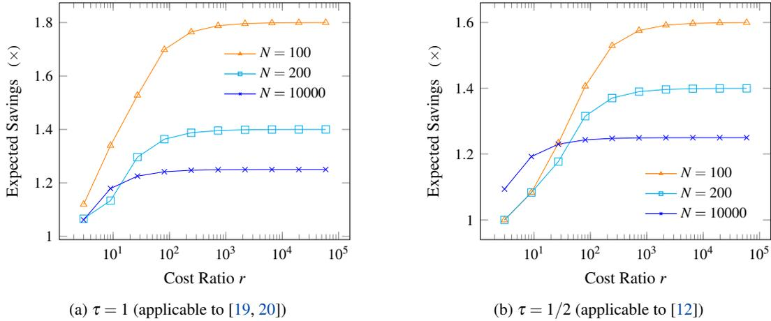
Figure 8: Bandwidth savings for BatchedCut protocols ( $\varepsilon = 2^{-40}$  and the check ratio  $c \geq 0.02$ )
