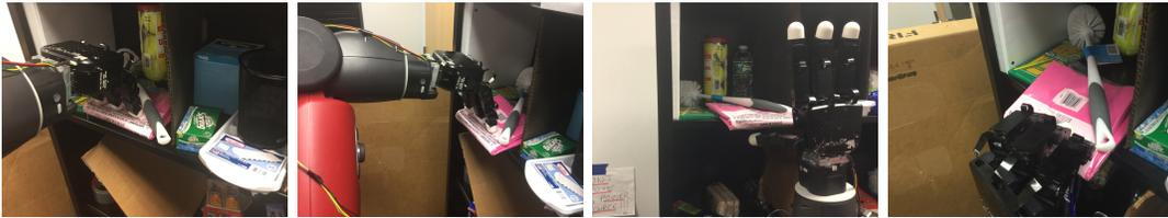
Fig. 2: The slide to edge manipulation process is illustrated above. After the object is dragged past the brim of the shelf, the hand is retracted and a pre-selected hand template is moved a set distance away from the brim of the shelf such that a compliant grasp will successfully grasp any object slightly protruding from the brim.
