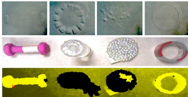
Fig. 1: Tactile imaging for four of the known ARC objects, along with their rgb and depth equivalents. As seen above, tactile imaging is fully capable of transmitting detail unavailable to traditional time-of-flight depth sensors.
