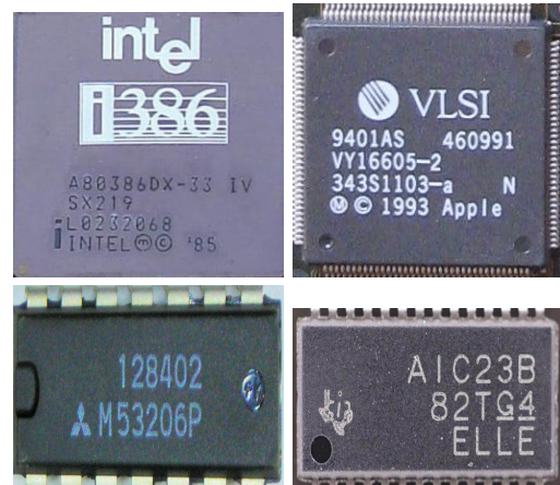
Fig. 1: We propose to learn deep embeddings from images of integrated circuits to retrieve, recognize, and verify them. Some instances from our dataset are shown.
