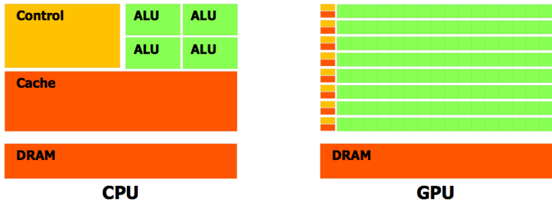
Figure 5: CPU and nVidia GPU basic architecture
